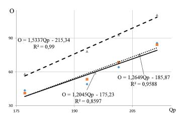
Figure 5. Effective set-up rate (O) when changing the operating modes of the compressor  $(Q_n, m^3/s \cdot 10^{-6})$ . Solid, dotted, dashed lines – design options I, II, III, respectively
