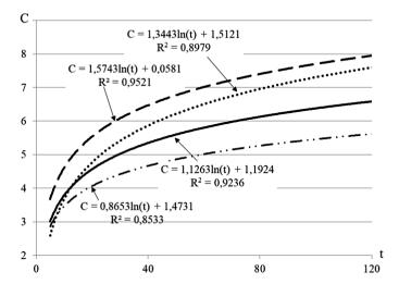
**Figure 6.** Dynamics of water oxygenation (C, mg/L). Solid, dotted, dashed lines – liquid supply by airlift ( $Q_y$ ,m<sup>3</sup>/s·10<sup>-6</sup>), respectively, 6.25, 7.72 and 22.86, dashed-dotted line – conventional aerator, (t, min) duration of aeration,
