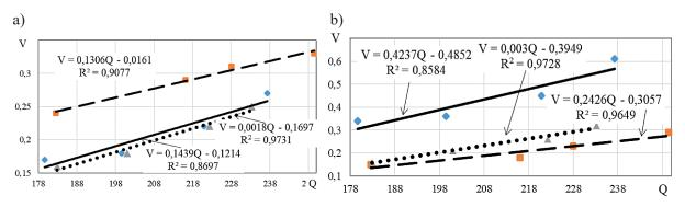
**Figure 3.** Velocity of air bubbles (V, m/s) in the mixing chamber (a) and the airlift column (b) depending on the performance of the set-up ( $Q_u$ , m<sup>3</sup>/s·10<sup>-6</sup>). Solid, dotted, dashed lines – respectively I, II, III options of the airlift design
